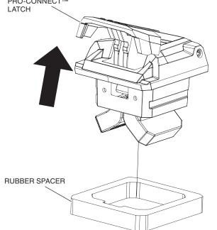
2. Insert the Pro-Connect<sup>™</sup> latch assembled with the rubber spacers in the Bed Rack installation square holes and secure them by using the Snap Rings.
