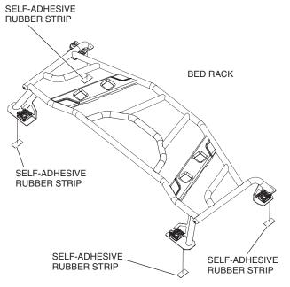
4. Make sure the Pro-Connect<sup>™</sup> latch levers are in the open position then locate the Bed Rack onto the Vehicle Bed by aligning each Pro-Connect<sup>™</sup> latch with his corresponding bed installation hole. Lock the Bed Rack in place by pressing down the four Pro-Connect<sup>™</sup> latch levers. To remove the Bed Rack from the vehicle, just lift the lever from each Pro-Connect<sup>™</sup> latch and freely remove the accessory.
